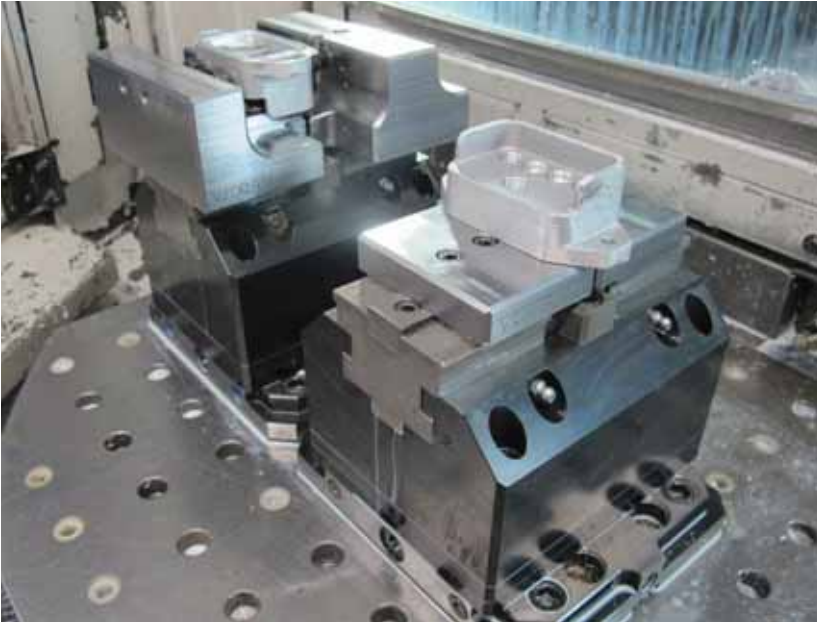
2 BSP-160 vices with special jaw connection, adapted to a jaw interface specified by the customer. The vices are mounted on a mechanical zero-point clamping system. Workpiece-specific jaws clamp the workpiece.
