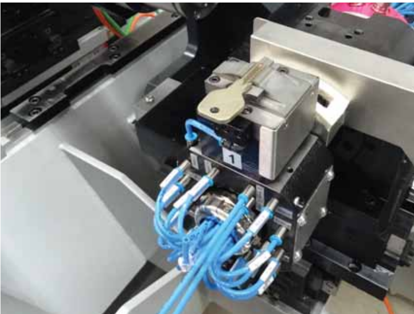
BSP-64 as a special vice in design according to customer requirements. The vice can be used either as a centric vice or as a fixed jaw vice.
