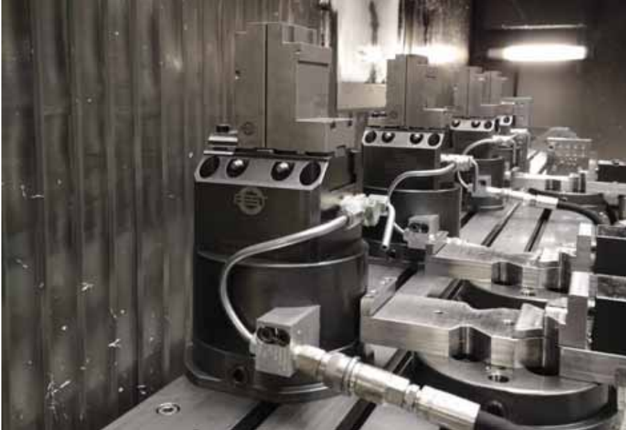
4 BSH-100-FR vices clamping a profile from the inside out. The vices have a spring return. Here the drawing WITHOUT tool.
