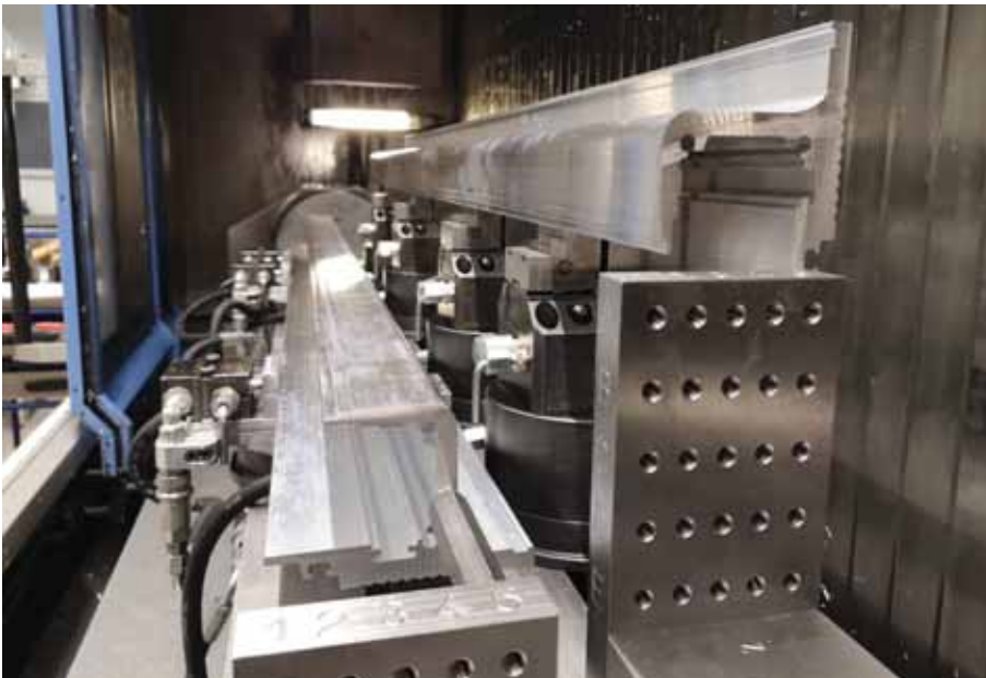
4 BSH-100-FR vices clamping a profile from the inside out. The vices have a spring return. Here the drawing WITH tool.
